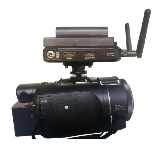
The transmitter is Horizontal installed and is mounted on the hot shoe of the camera through the bottom 1/4 threaded hole
