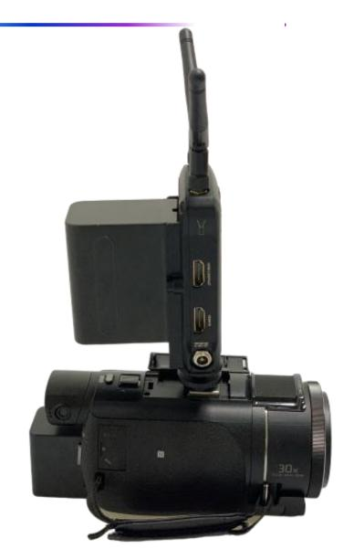
The transmitter is installed vertically and is mounted on the hot shoe of the camera through the bottom 1/4 threaded hole
