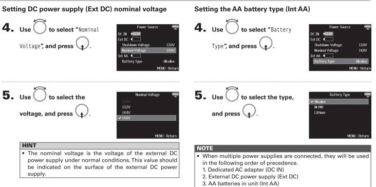
• The voltages of each power supply are shown on the display.
